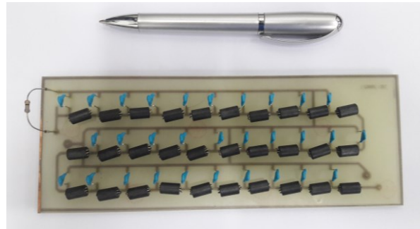
Figure 6. The HNLTL assembled on a PCB.
